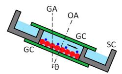
FIG. 1. Schematic diagram of the sample cell (side view): SC, stainless steel cell; GC, glass cover slip; GA, vertical (gravity) axis; OA, optical axis;  $\theta$ , tilt angle of the sample cell; red particles, large polystyrene latex spheres forming a monolayer crystal on the bottom glass substrate; blue particles, smaller diffusing particles on top of the colloidal crystal; arrow, direction of the force *F* acting on the diffusing particles.
