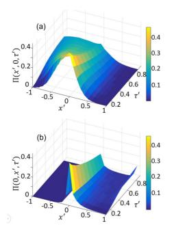
FIG. 6. (a) 3D plot of the measured reverse TPDF  $\Pi(x',0,\tau')$  as a function of x' and  $\tau'$  under a tilt force  $F/F_T = 3.7$  along the [1,0] crystalline direction. (b) 3D plot of the measured forward TPDF  $\Pi(0,x',\tau')$  under the same condition as that in (a).
