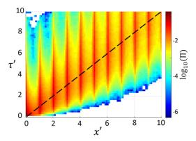
FIG. 3. 3D plot of the measured FTPDF  $\Pi(0, x', \tau')$  under a tilt force  $F/F_T = 7.4$  along the [1,0] crystalline direction. Here the normalized distance  $x' = X/\lambda$  and delay time  $\tau' = \tau/(\lambda/v_d)$  are used in the plot (see text for details about their definitions). The values of  $\Pi(0, x', \tau')$  are color-coded in log scale for better visualization. The black dashed line indicates  $x' = \tau'$ .
