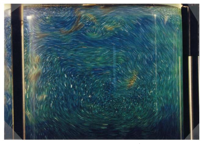
FIG. 4. (Color) A streak image of the TLC spheres taken in the A = 1 cell at Ra= $2.6 \times 10^9$ . Cold eruptions are brown; green and blue regions are warmer. The displayed region covers top 2/3 of the convection cell and its dimension is approximately 20 cm  $\times 14$  cm.
