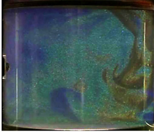
FIGURE 2. Flow visualization image of small TLC spheres taken in the \Gamma = 1 cell at Ra = 3.7 \times 10^8 and Pr = 5.3 . Cold eruptions are brown; green and blue regions are warmer. The displayed region covers the entire convection cell and its physical dimension is approximately 10 \times 10 \text{ cm}^2 .
