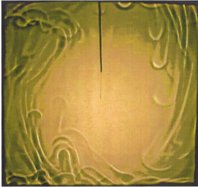
FIG. 2 (color). A shadowgraph showing the spatial distribution of thermal plumes in an aspect-ratio-one cell ( H = 15 cm) filled with dipropylene glycol ( Pr = 596 ). The picture is taken at Ra = 6.8 \times 10^8 .
